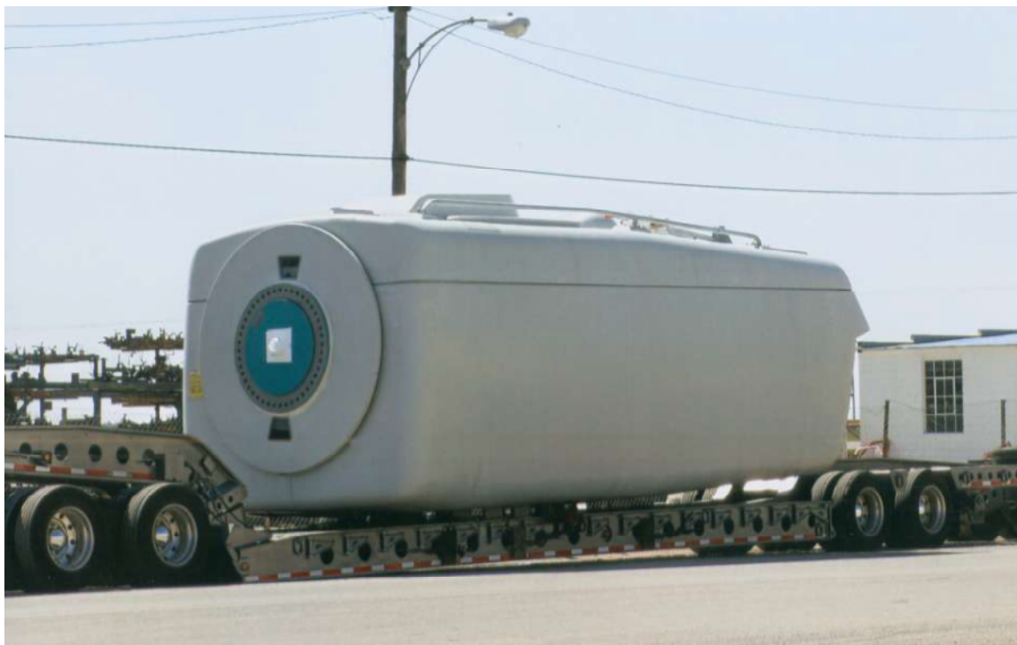
Figure 2-3: Nacelle transportation. (Sri, S., 2011)
