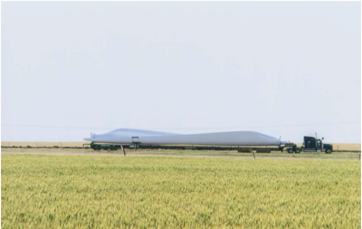
Figure 2-2: Blades transportation. (Sri, S., 2011)
